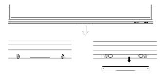
2. Insert the WiFi module fully into the monitor along the direction of the arrow.
